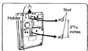
To temporarily place the handset down during a conversation, hook as shown.
